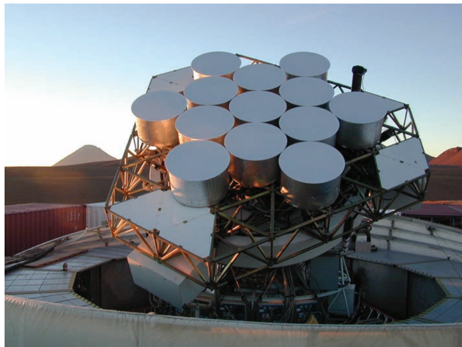
Fig. 1. The CBI. For the polarization observations, the 13 90-cm Cassegrain antennae were arranged in this hexagonal close-packed configuration on the rotating, alt-az mounted platform, with six adjusted to be sensitive to righthand circularly polarized radiation and seven to lefthand circularly polarized radiation. By correlating the signals from the antennas in pairs, 78 interferometer baselines are obtained ranging in length from 1.0 to 3.5 m.
